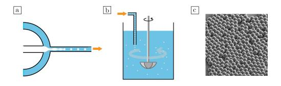
Figure 1: (a) Producing uncured droplets with a microfluidic chip. (b) Droplets are being stirred in a beaker to be cured into particles or capsules. (e) SEM image of nearly neutrally buoyant particles [1].
