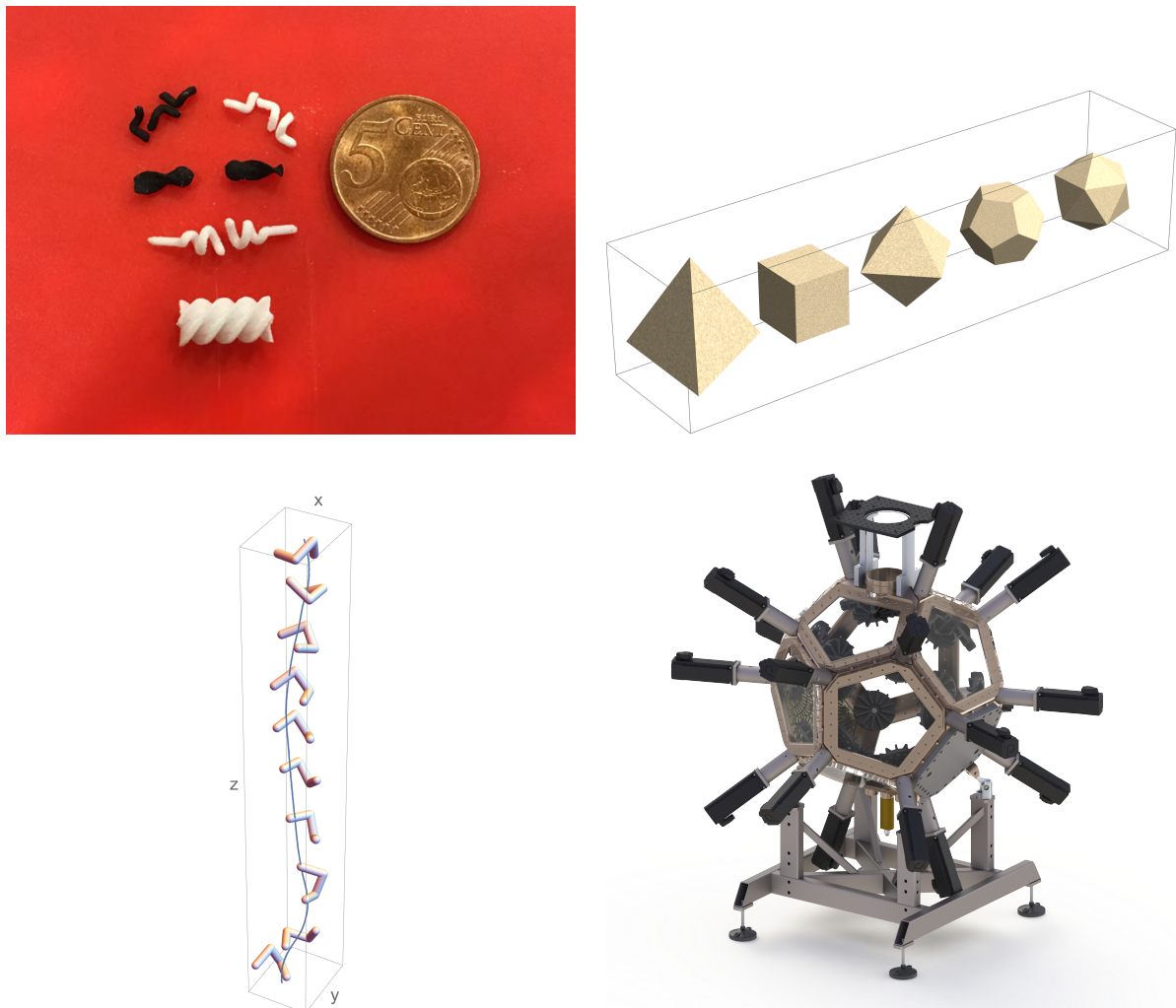
Figure 1: Top-left: Examples of some particles. Top-right: rendering of possible 3D-printed particles (platonic solids). Bottom-Left: typical chiral particle. Bottom-right: Dodecahedron with a volume of \approx 210 L.
