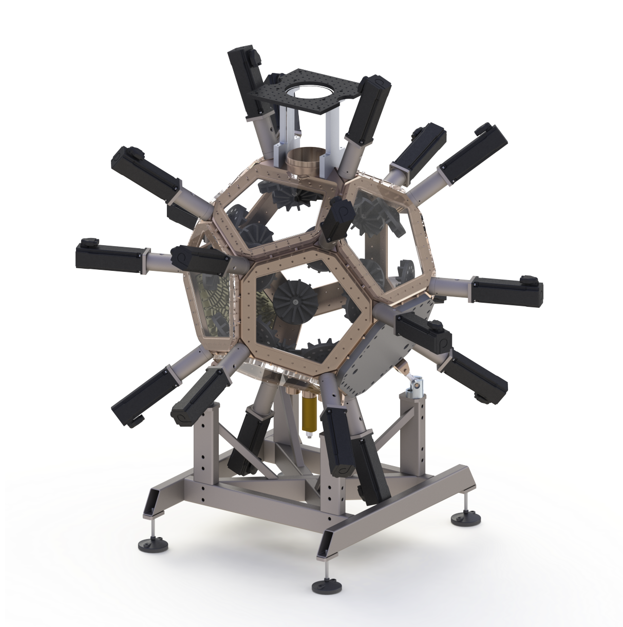
Figure 1: Dodecahedron with a volume of \approx 210 L.
