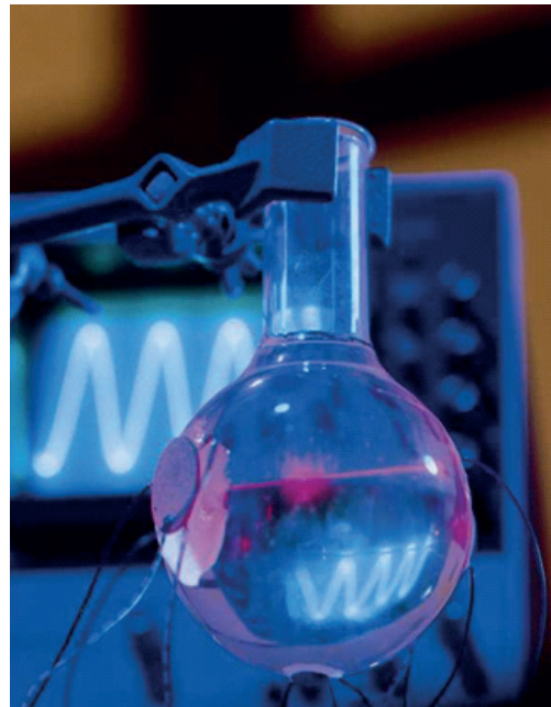
FIG. 1: Setup for single bubble sonoluminescence: Piezos are glued to a flask filled with water. They excite a standing acoustic wave in which the light-emitting bubble is trapped. This setup has its resonance frequency at about 20 kHz. Photo taken by Rüdiger Tögel, Physics of Fluids, Twente, 2000. I also chose this photo as cover page for the booklet with my inaugural speech.
