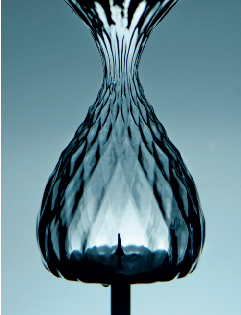
FIG. 17: Void forming after the impact of a non-axisymmetric disk on a water surface. Oscar Enríquez called this photograph the “pineapple”. Figure taken from [149].
